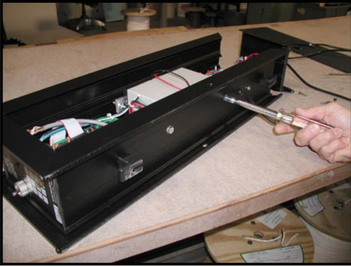
Move the battery charger power cord out of the way and remove the first battery clamp bolt.
