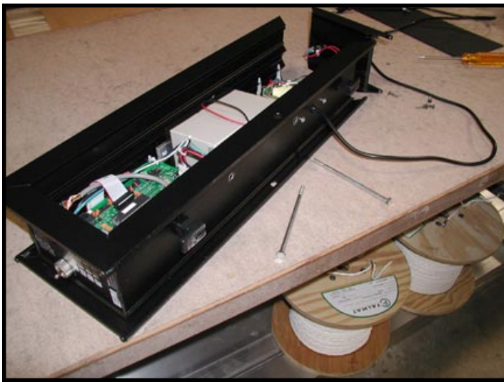
Battery clamp bolts removed.
