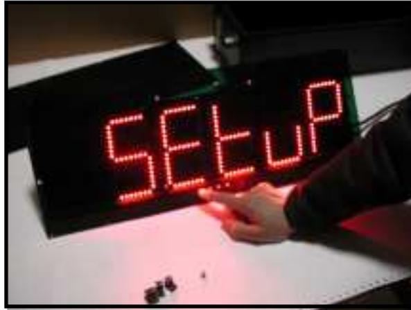
Push the Menu (left hand button) to access the SETuP menu and make any necessary changes.
