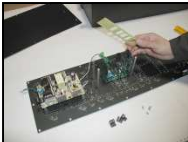
Remove the module hold-down plate.
