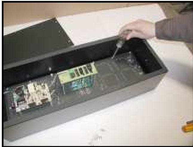
Using a 3/8" nut-driver, remove the 16 display board nuts.
