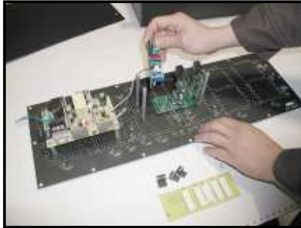
Plug in the power supply card.
