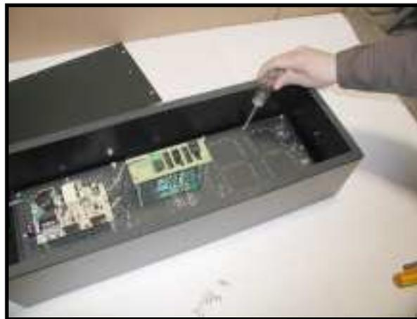
Install the 16 nuts on the studs.
