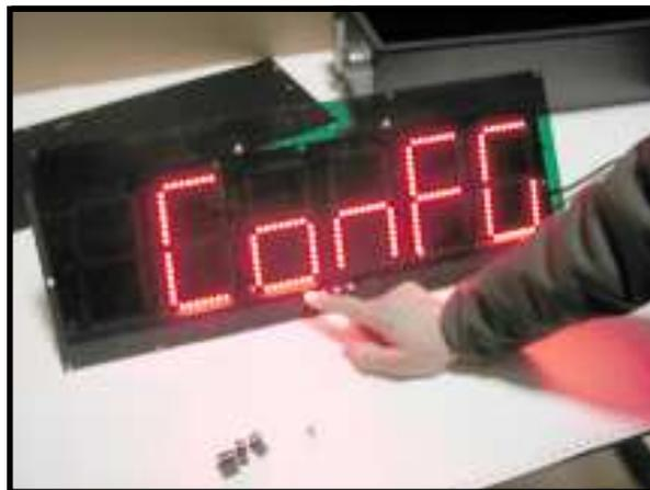
Push the Menu (left hand button) to access the ConFG menu and make any necessary changes.
