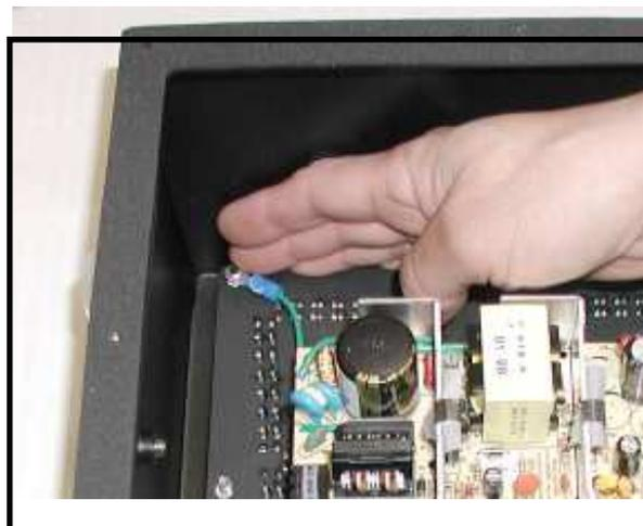
Be sure the green jumper wire is installed on the stud under the nut as shown.
