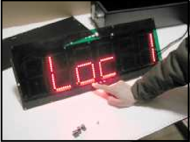
Push the Menu (left hand button) to access the Loc-1 menu.
