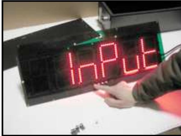
Push the Menu (left hand button) to access the InPut Menu and make any necessary changes.
