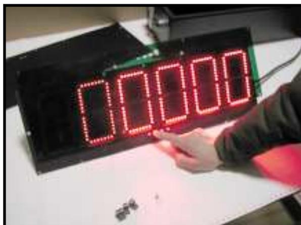
With all "0"s showing, the Loc-2 to Loc-4 menus are completely unlocked.
