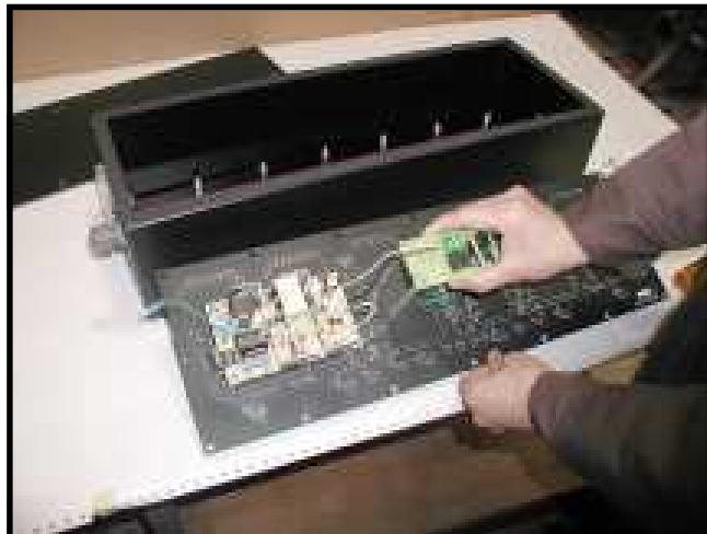
Remove the display board from the enclosure.
