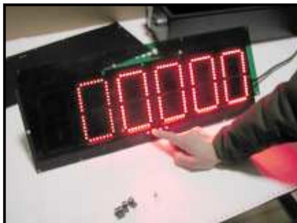
With all "0"s showing, the Lock-1 menu is completely unlocked.
