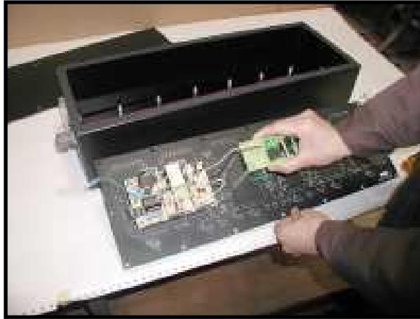
Place the display board assembly into the case over the 16 studs.
