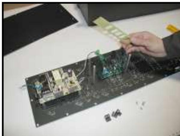
Remove the module hold-down plate.
