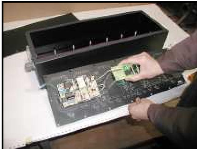
Remove the display board from the enclosure.
