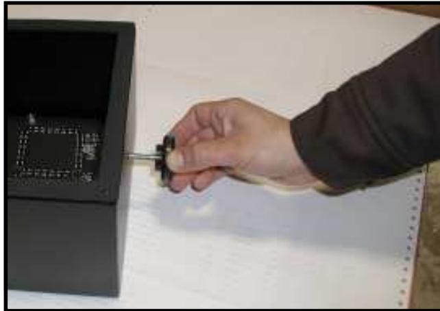
If installed, unscrew the hand knobs
