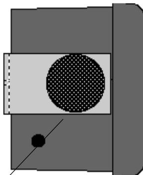
**NOTE:** Plastic plugs are provided to seal unused bail clamp screw holes.
