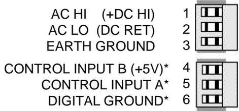
\*Note: Non-isolated external control inputs A and B are menu selectable in the menu item "Setup". Input B is jumper selectable for either a control input or +5V output.
